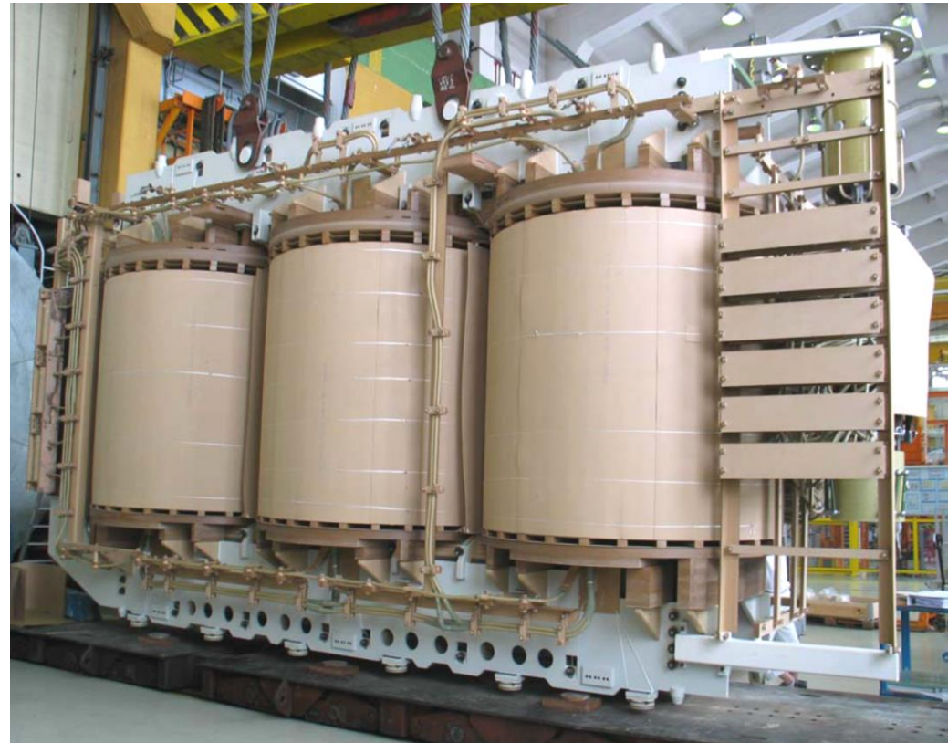
Conventional 400 MVA Transformer
